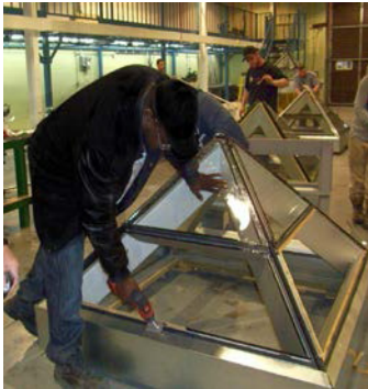
Apprentice glazing Alumicor skylight
